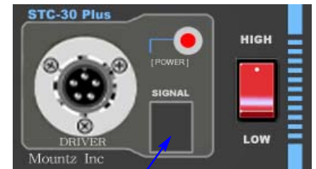
Plug cable from Scout into transformer
