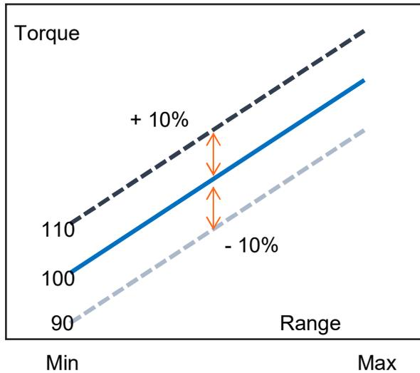
A periodical torque calibration is required to keep the accuracy of fastening quality.
