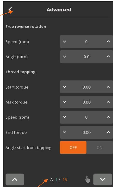
Parameters listed on A and B pages for each Preset from 1 to 15
