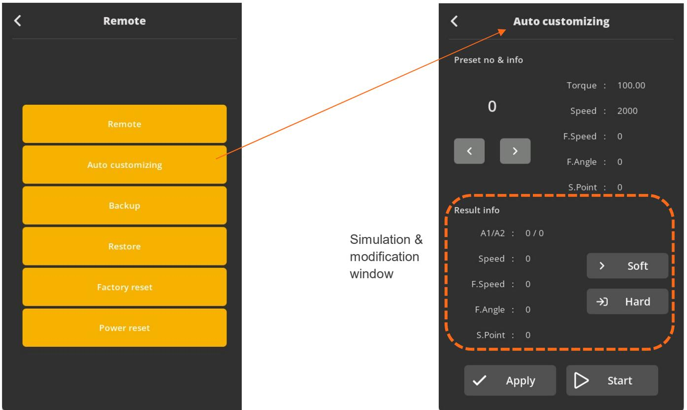
EC and ECT tool has the auto speed setting feature against torque setting to minimize over torque by speed shock. This auto speed is safe speed on the hard joint condition. On the real application, this setting can be changed manually. Auto customizing feature provides optimized parameter settings for saving cycle time on the real application.
