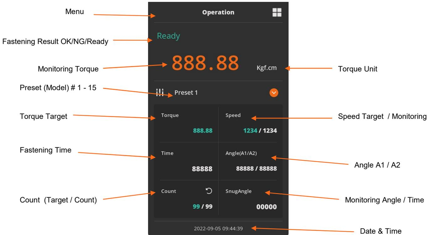
Operation screen is a default window when the controller power ON.
