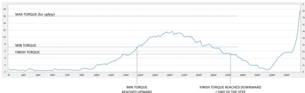
It is not the case in the chart (on prior page), but the tapping torque can be higher than the target torque (tapping in metal sheets, for example)
