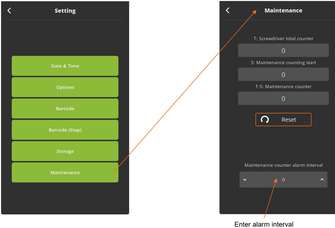
This step will trigger a banner stating maintenance interval is needed.
