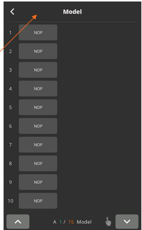
They are 15 sequencing models of 20 steps with assignable tightening program batch counting and logical IO management.
