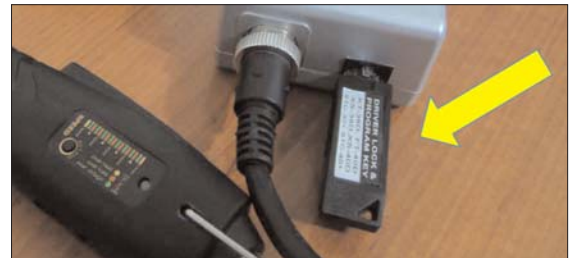
To adjust the settings the Program Lock Key must be plugged into the STC40 or FT-30D Mini Transformer.
