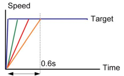
The Soft Start button is “wrap around” button meaning you can toggle through the settings continuously by pressing the button (OFF - 0.2s-0.4s-0.6s).
