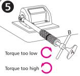
If the torque is too low, hold Bar A and Bar B and turn clockwise together; if the torque is too high, hold Bar A and Bar B and turn counterclockwise together.
