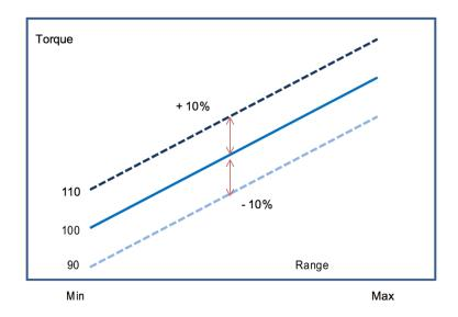
Standard test condition on factory calibration used by Mountz
