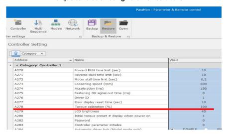
When the reading on the torque meter master is lower than the setting on the tool, increase the calibration value more than 100(%) which is basic on production. To increase the output torque 5% more, key in 105(%). The calibration value works through whole range of torque. It will be refreshed and stored in the memory of the tool so it can be still effective when using the tool on another controller.
