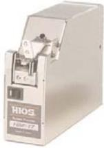
**Screw presenters** are small, tabletop devices used to organize and automate work areas and production cells. Screw presenters make assemblers and the assembly process more efficient by mechanically presenting a screw to a fixed pick up point. The inexpensive screw presenter is an alternative tool instead of the cumbersome and very expensive screwfeeder systems.
