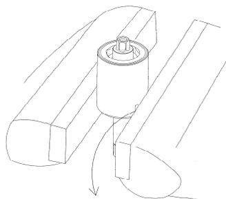
2. Loosen (CCW) the torque adjustment screw all the way up to the minimum. Remove the greasing screw (plug) and with the use of a syringe, remove the oil completely. Turn the anvil back and forth one turn to release any oil excess. Use syringe to remove any oil remaining in the unit.
