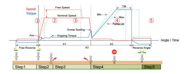
\*Fastening process of the screws is divide into five steps, controls each step with presets and advanced functions.
