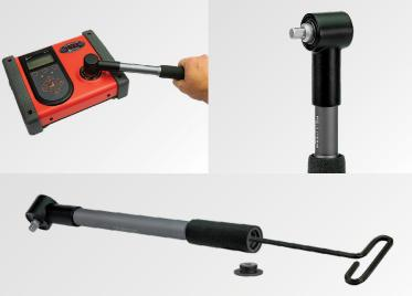
Tamper-proof internal adjustment. No external adjustment scale—must be preset using a torque analyzer.
